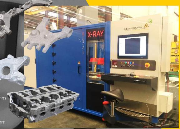
Thanks to its C-Frame technology, **XC01-1100** reaches all necessary inspection areas without any dead-zones. High performed fully controlled servo axes makes it one of the fastest inline casting inspection systems. Based on integrated automatic type recognition, **XC01-1100** can be used for different casting parts without any delays. When production changes to a different product, the product specific inlet plate has to be replaced within extremely short time.
